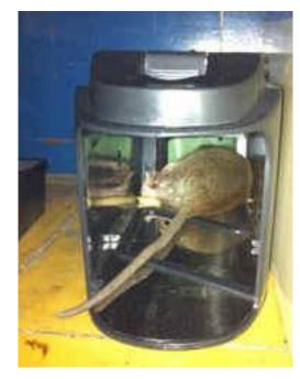
trap through having a piece of bait inside. When the mouse (or rat) steps on a special plate inside the trap, it completes an electronic circuit, which sends a high voltage current through the animal, killing it instantly and cleanly.
