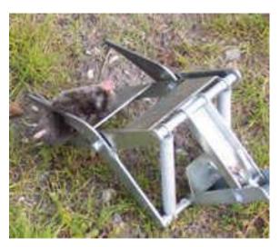
One of the best mole traps is the Wire Tek 1001 EasySet Mole Eliminator Trap. This trap works by having two powerful scissors like mechanisms that are inserted into the top of a mole tunnel. The device is then primed by depressing the setting level by foot.
